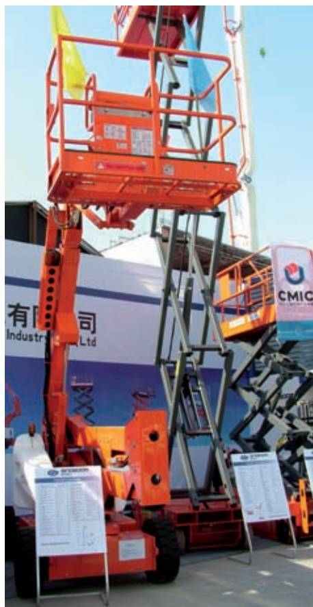
Chinese manufacturer Sinoboom showed a new 41.6 m platform height telescopic boom and this electric 15 m articulated boom at bauma china.
