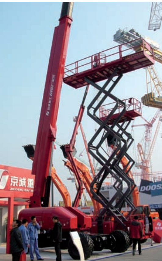
A new 42 m telescopic boom and 13 m rough terrain scissor were launched by Beijing Jingcheng.
