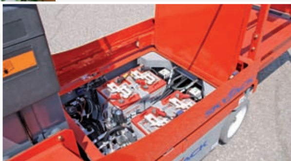
The design of the base of the Skyjack's SJ 12 gives unobstructed access to batteries and other components for easy maintenance.
