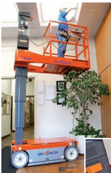
The design of the base of the Skyjack's SJ 12 gives unobstructed access to batteries and other components for easy maintenance.
