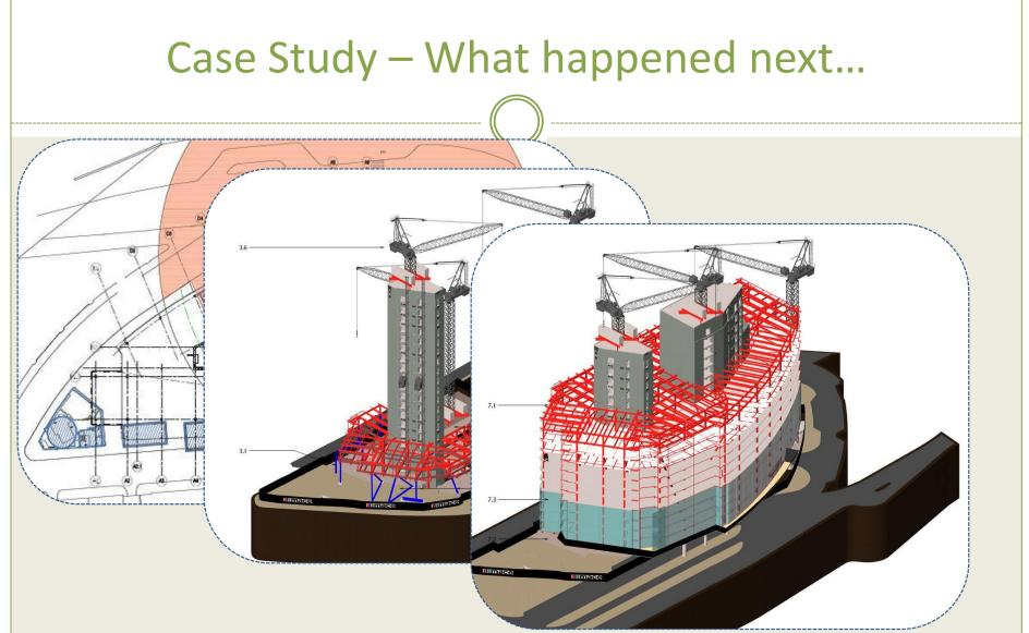
• With over 10 operations, including erections, climbs, dismantles and jib extensions / reductions only three operations required a mobile crane
