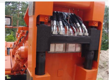
System 2: Fully hydraulic QuickConnect System
