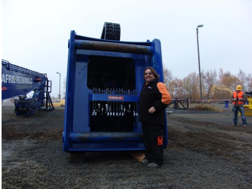
OQ180 QuickConnect Adaptor with up to 30 connectors/couplings
