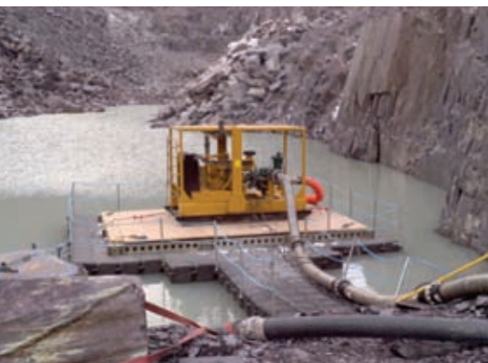
A Pioneer 150CM high pressure pumpset working at the Welsh Slate Penrhyn Quarry.
