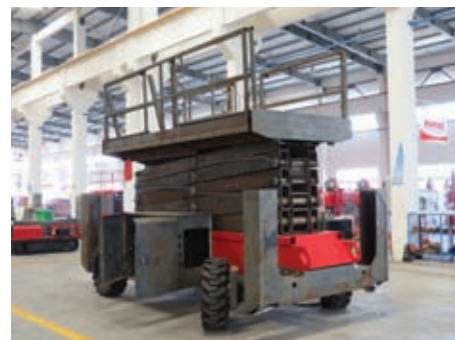
This is an 18 m rough terrain scissor being developed by Mantall. It will be powered by a Kubota engine.
