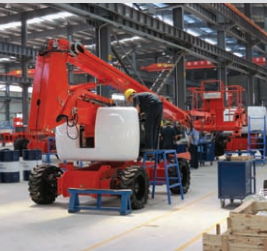
Booms under production at Sinoboom's facility. A paint booth is currently under construction.
