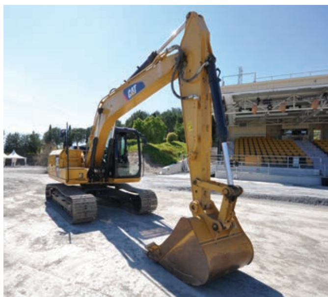
The 313F L GC excavator features new Cat Connect monitoring systems
