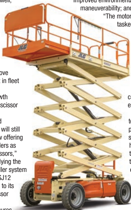
JLG offers three series of electric scissors – the ES, RS and LE series.
