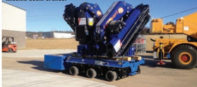
PSC's SPMT 600 shown transporting knuckle boom cranes.
