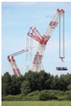
CC 8800 Twin at an all terrain crane lifting
