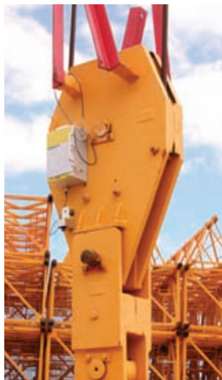
HookCam gives operators a live view from their hook's perspective.
