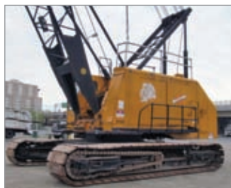
1980 Manitowoc 3900 w/ Lattice-Boom Crawler Crane
