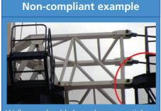
Walkways should always have gaps tighter than 200 mm. The gap showed in the picture can be dangerous for the operator.
