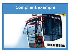
3. Gaps in walkways: wide gaps can cause falling hazard.
