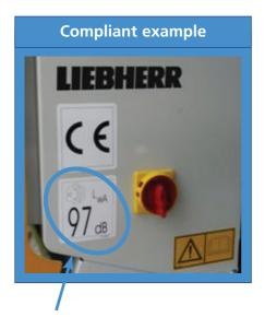
The sound level is printed in decals. The sound power level is generally positioned at the bottom of the crane and in the crane's upper part
