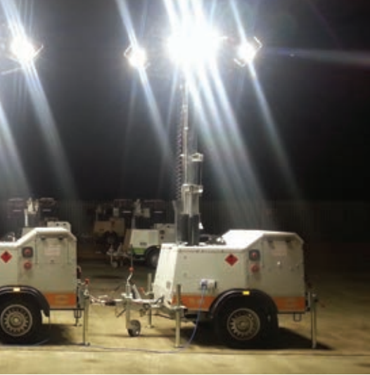
Morris Site Machinery said it planned to showcase its SMC TL-90 LED lighting tower, featuring five 240 W LED lamps and a 1500 rpm Kubota engine
