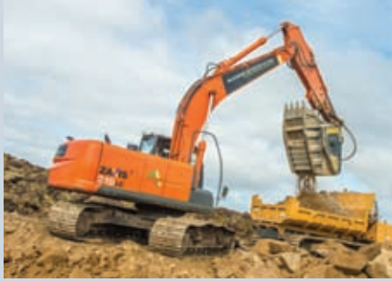
An MB Dig A Crusher BF90.1 crushing bucket, teamed with a Hitachi ZX210, is supplying 30 tonnes of material per hour for use for paths and roads in remote parts of Scotland
