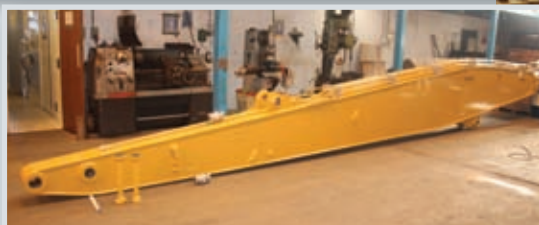
The boom is almost ready for installation - the main boom, intermediate and upper dipper arm await the carrier's completion
