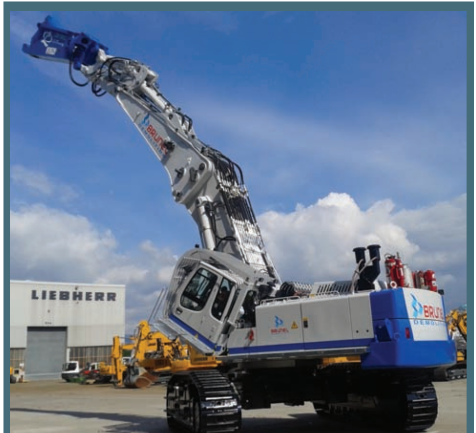
Liebherr has modified an R 974 C demolition specification excavator to allow it to carry a 13,410 kg (29,500 lb) La Bounty MSD 7500 R shear for French contractor Brunel Demolition that will find use during the demolition of power stations. In addition to the usual tilting cab and extending undercarriage, the new machine features a mechanical quick coupler system for the boom that allows an attachment change in just 10 minutes. Liebherr says that the demolition versions of its excavators will be delivered with a Stage IIIA/Tier 3 engine until the end of 2015.
