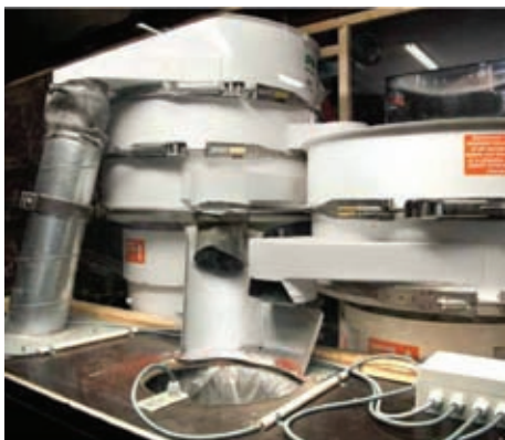
An efficient filter system is at the heart of the system that separates pollutants from the abrasive agent following coating removal
