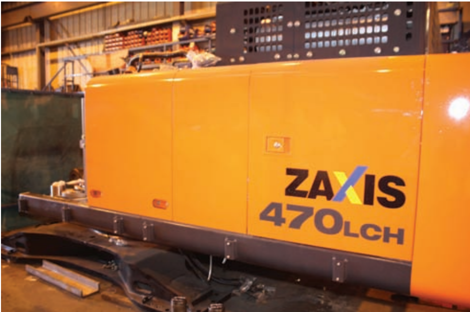
Work has begun at Kocurek's facility to convert a Hitachi ZX470 carrier to turn it into a true multicarrier to allow it to mount the multiplicity of booms planned by Kiesel
