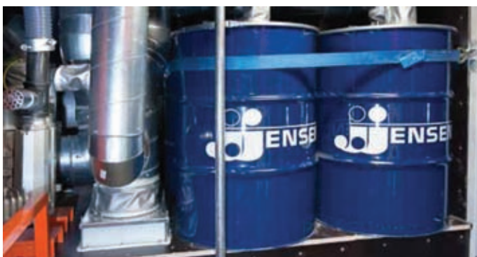
An efficient filter system is at the heart of the system that separates pollutants from the abrasive agent following coating removal
