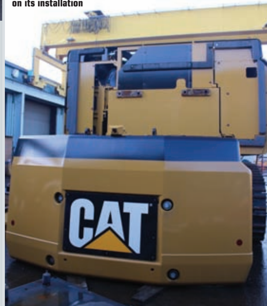
The carrier will feature a dismountable additional counterweight. Work has begun on its installation
