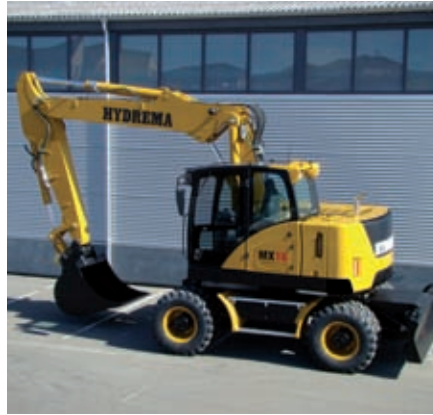
The 19 tonne class MX18 from Hydrema, part of a new Stage IIIB-compliant wheeled excavator range
