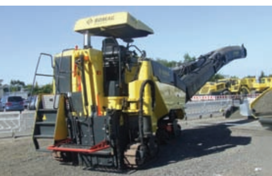
Bomag's new BM1000 is a 257kW, Tier 4 Final/ Stage IV-compliant milling machine
