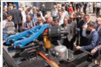
Goldhofer's PST/ES-E 24 with hydraulically adjustable track width was introduced as well as its MPA Axle Technology for SPMTs.
