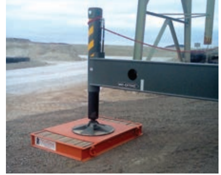
A Saskatchewan crane company bought a new Terex Explorer AT and rigged it using C-Channel reinforced timber matting.
